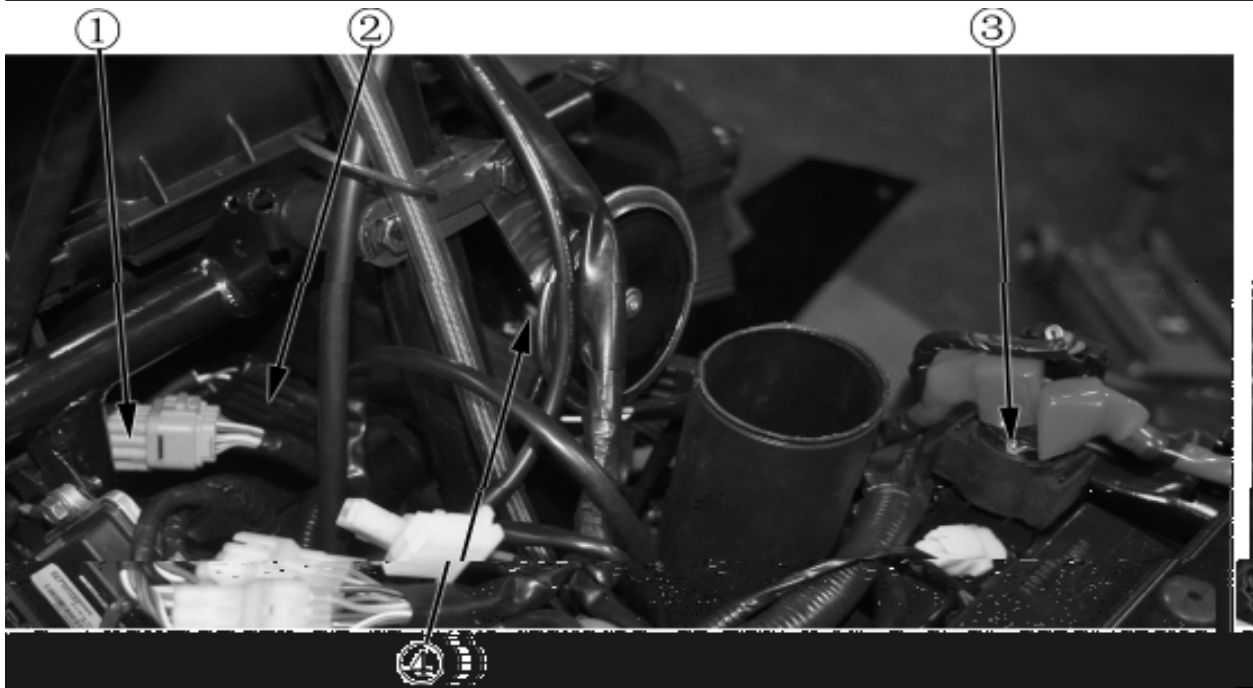
1.Connector, auxiliary cable 2.Connector1, oxygen sensor 3. Starter relay 4.Connector, horn
